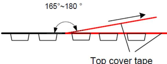
The force for tearing off cover tape is 10 to 130 grams in the arrow direction.
